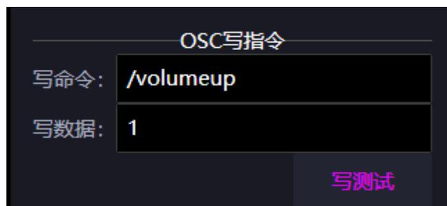
Click 'Write Test' to send a command to the target device to test if it is under control. After clicking, the "Test Results" below can clearly show the data and type sent, the target IP address, port, and the completion status of the transmission.
