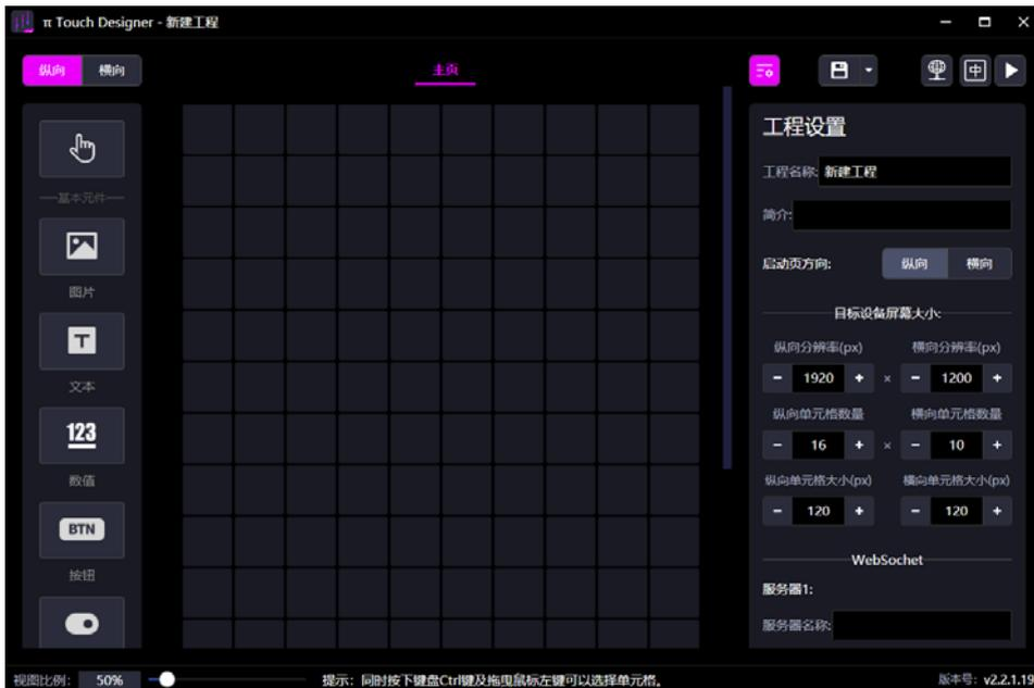
Click on any square at any position, set the starting position, number of rows, and number of columns of the cell on the right side, and click add panel after setting.
