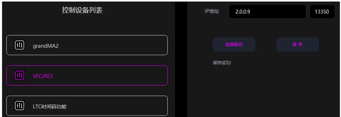
IP address input box, enter the IP address of the VFC/RES video server.
