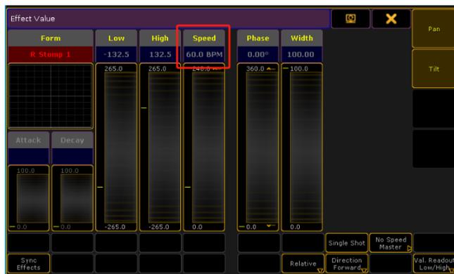
If the lighting program needs to follow the BPM at a steady pace, the original Speed BPM must be a multiple of 60, 1/8, 1/4, 1/2, 1, 2, 4, 8 times.
