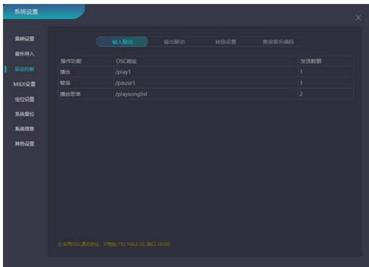
This page is the input linkage in linkage control, which contains the OSC address of the play and pause keys, and is the input address of the OSC protocol; the sent data is the linkage data of the OSC protocol. The output linkage needs to be linked with the input data.
