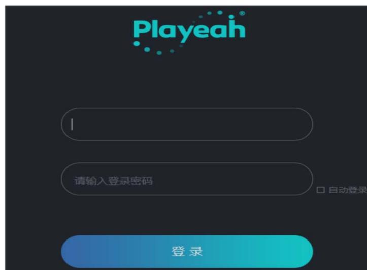
Users can enter the system and start using it by entering their account and password. If the "automatic login" option is selected, the system will save the last entered account and password and automatically log in after power on.
