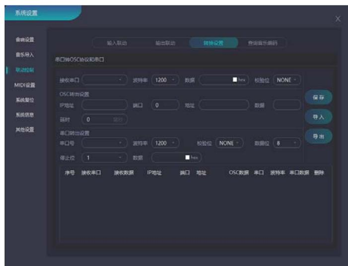
This page is for conversion settings. **串口转OSC协议和串口** In the system, the serial port is connected (this serial port is the serial port for external input devices). After the connection, this serial port is converted to OSC protocol or 485/232 protocol serial port.
