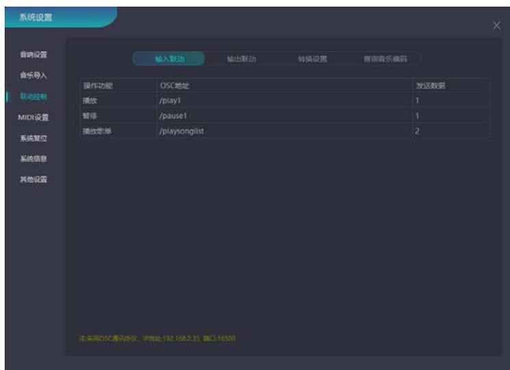
This page is for linkage control. Space Pro adopts OSC control protocol, which can communicate and control with external devices such as video and lighting, allowing video playback or lighting effects to change with the music.
